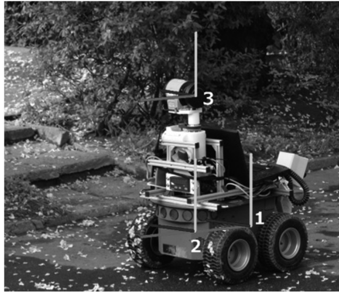
Fig. 1. Small Mobile Mapping System with three coordinate systems: 1) mobile robot odometry – global, 2) IMU, 3) 3D laser scanner
