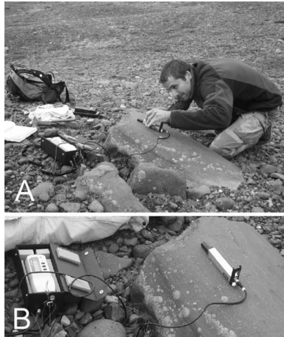
Text-fig. 3. Measuring rock surface micro-roughness of glacially-abraded boulder (A); Handysurf E35-B profilometer (B). Phot. A.Tittenbrun
