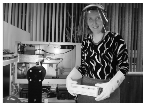
Fig. 6. Xenon lamp in a specially designed for testing luminaires and special measures of protection in the form of masks and gloves [7]
