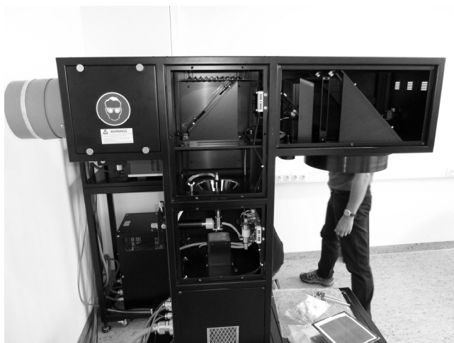
Fig. 2. The interior of „Super solar simulator” [Heiholtz Center in Berlin]
