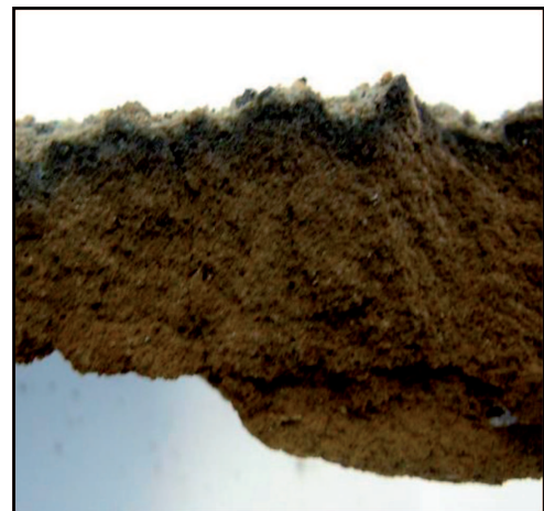
Fig. 5. Refractory material based on MgO
