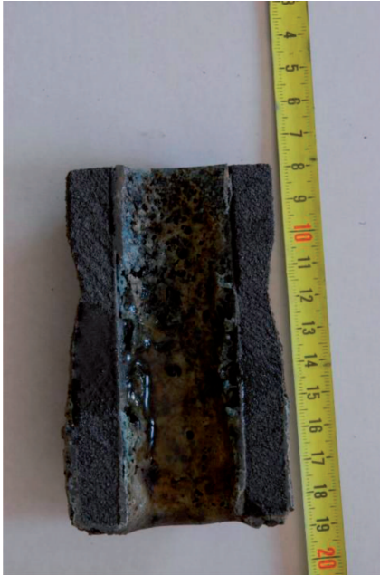
Fig. 6. Deposits in the bottom part of SEN (glassy phase is an added resin for structural stability)
