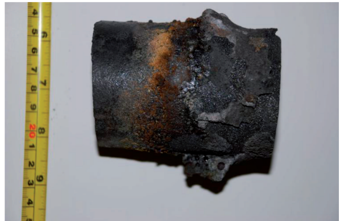
Fig. 4. Solidified cover slag on the thermocouple protective shroud
