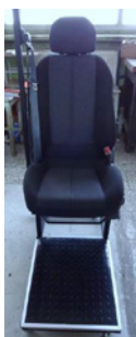
Car seat with headrest and seat belt to demonstrate a correct fastening of the seat belt
