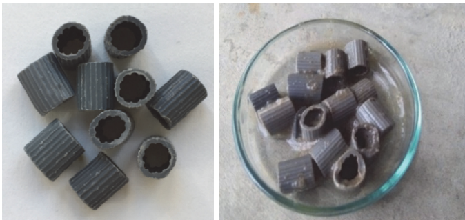
Fig. 2. The carrier EvU-Perl from Nowa Wieś WWTP (without and with biomass) (own photography)
