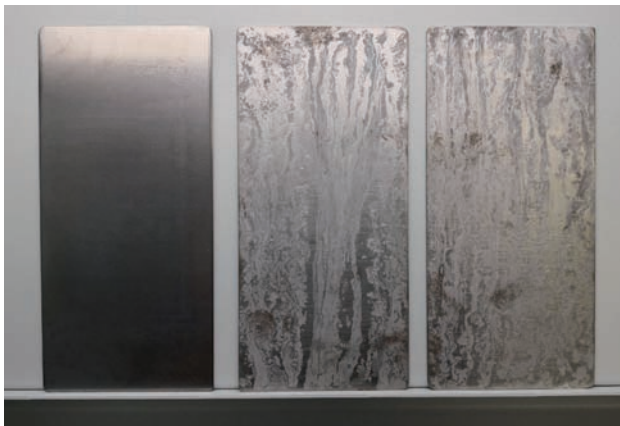
Fig. 3. CR4 steel calibration plates before and 48h after testing (etched) [Author's own elaboration]
