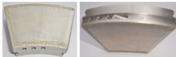
Figure 11: Bearing pad with the microrelief and the additional strips of the surface microrelief.
