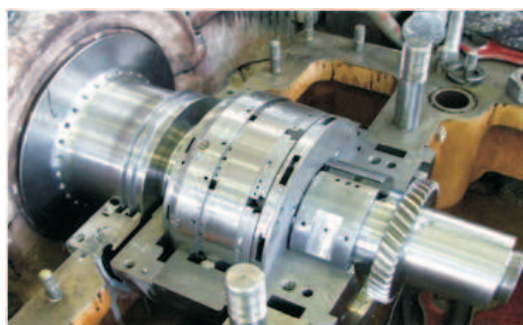
Figure 13: Journal-Thrust Bearing PDU –120/260 for Modernized Turbine 103JT.
