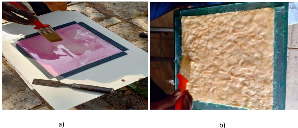
Figure 4. a) Manufacturing of plain epoxy composite, b) Manufacturing of WTNSFs reinforced composite.
