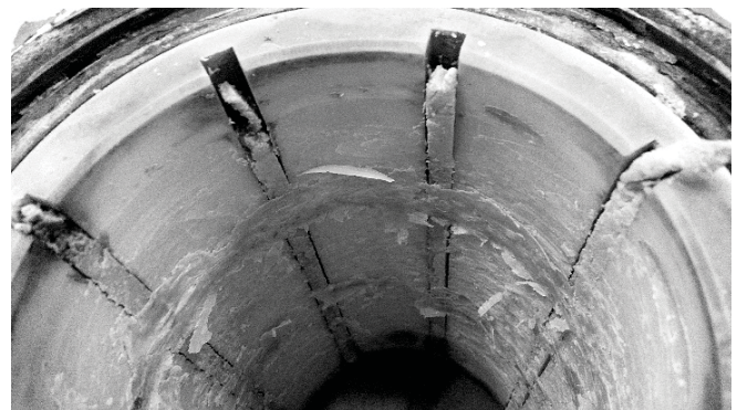
Fig. 1. Elastomer bush melted during the laboratory test. Test conditions: load: 0.2 MPa, speed 10 rev/s, water flow 0 L/min.
