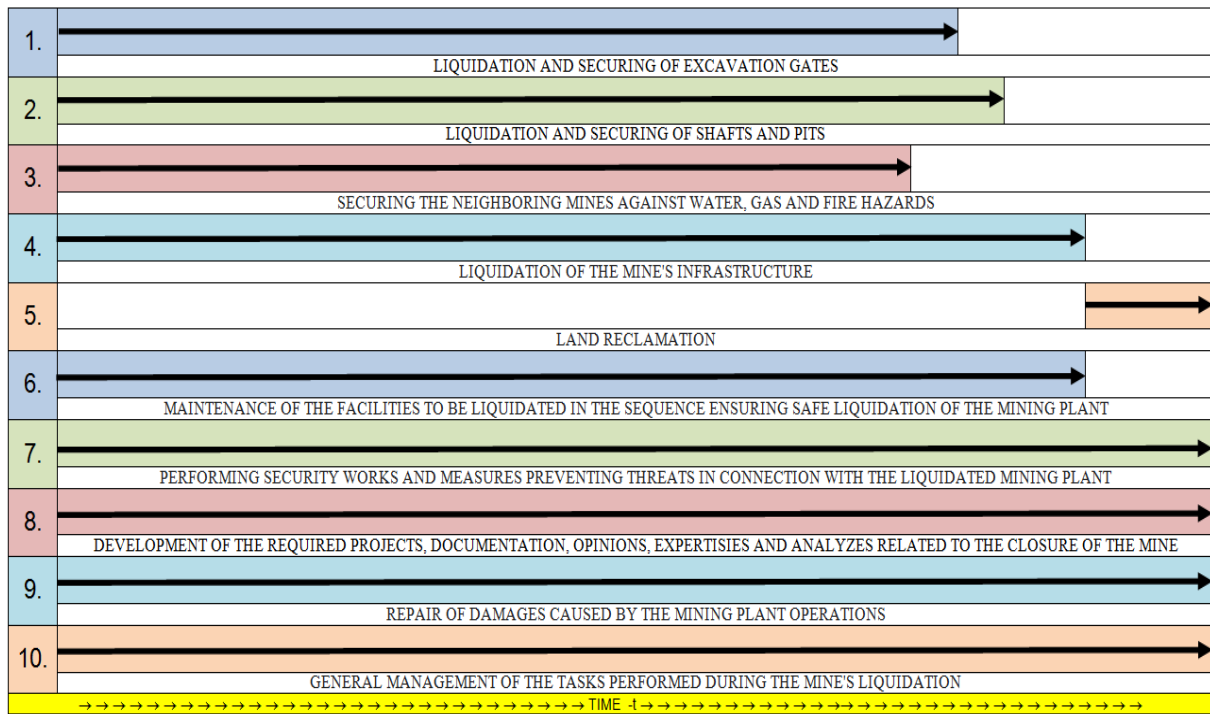
Figure 4. A schedule of the processes of complete mine liquidation in SRK S.A. Source: an own study.
