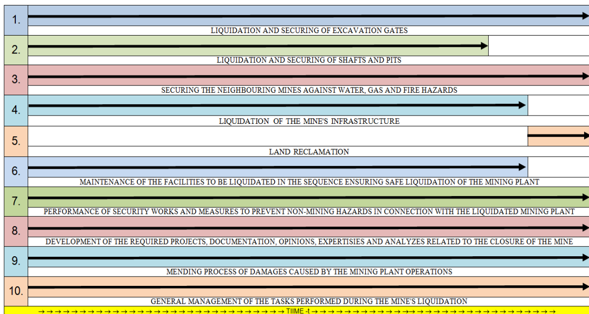
Figure 5. A schedule of the mine liquidation processes in SRK S.A. with further use of the pumping station. Source: an own study.
