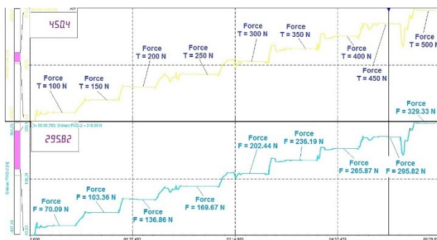
Fig. 5 Records of the monitored forces T [N] and F [N] in the environment of the DEWESoft X2 SP5 software during the experimental test on the measuring device
