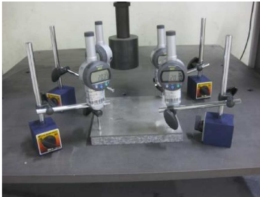
Fig. 2. A view of the test setup for compressibility measurement.
