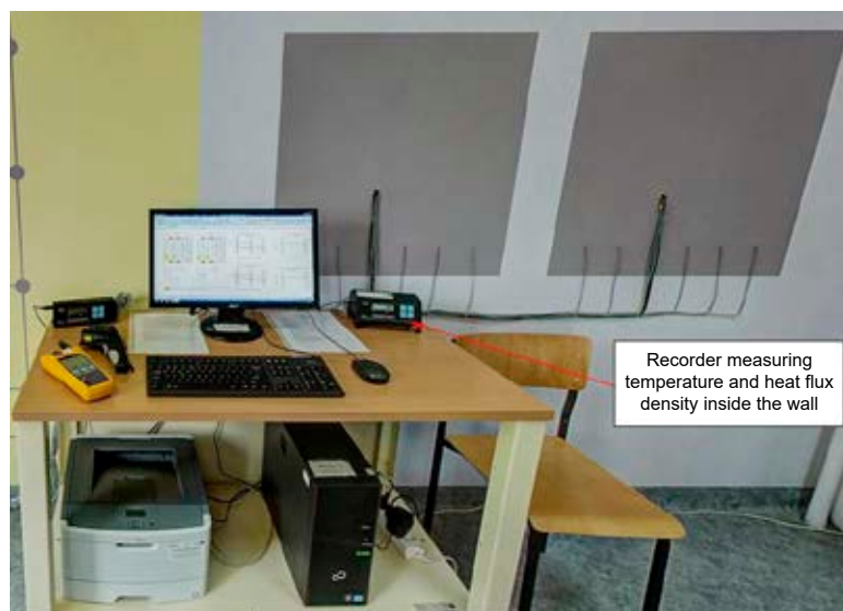
Figure 10. Station for measurement of temperature and heat flux density inside the wall
