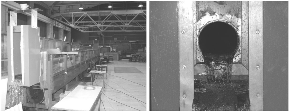
Fig. 3. Laboratory model of a single storm sewer pipe
