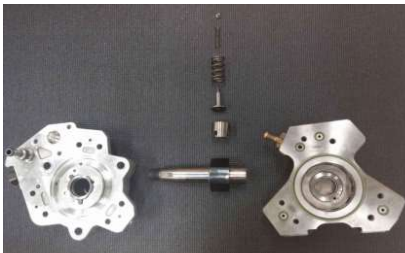
Fig. 2. Research object –the common rail pump Bosch type CP3S3
