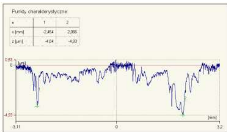
Fig. 6. Profile shows wear of the eccentric shaft CP3S high pressure pump at the point of cooperation with the sealing lip of the pump housing.
