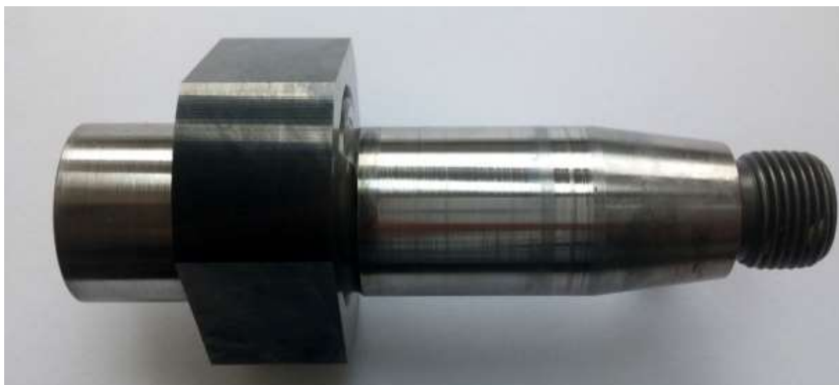
Fig. 3. Signs of wear on the pump shaft
