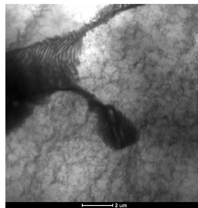
naroże próbki – ferryt corner of a sample – ferrite + pearlite
