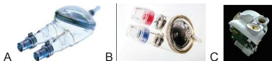
FIG. 1. Pulsatile heart prostheses: A - BerlinHeart EXCOR [3], B – ReligaHeart EXT [2], C – CARMAT TAH [4].
