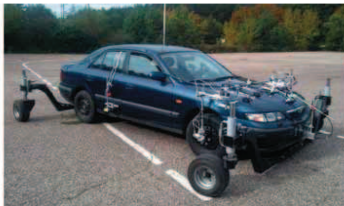
Fig. 5. Vehicle equipped with skidcar system and dynamic parameters measure sensors
