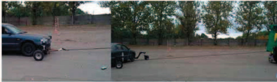
Fig. 4. Pull experiment for evaluation of longitudinal and lateral friction
