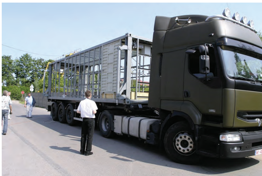
Fig. 2 The chassis and frame of container – final enclosure of the mobile laboratory (photo Paweł Włodarczyk WITPiS)
