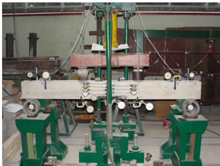
Fig. 2. The test machine and RC beam during testing ( own research )
