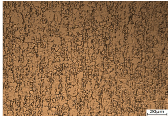
Fig. 7. Microstructure of titanium Ti-6V-4Al ELI specimens prior to forging
