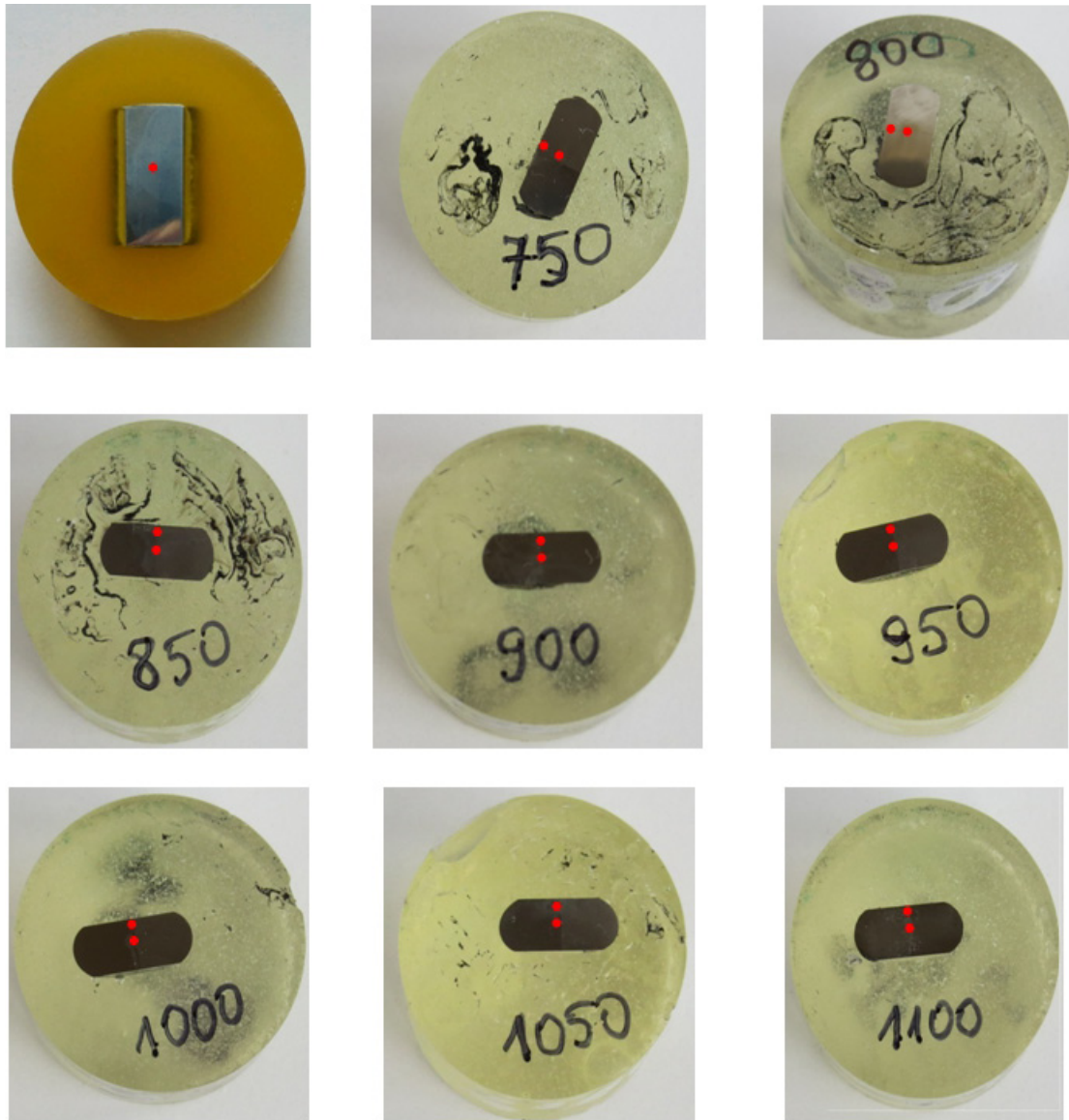
Fig. 4. Metallographic specimens for microscopic examination; red colour marks zones examined for micro-structure quality and hardness
