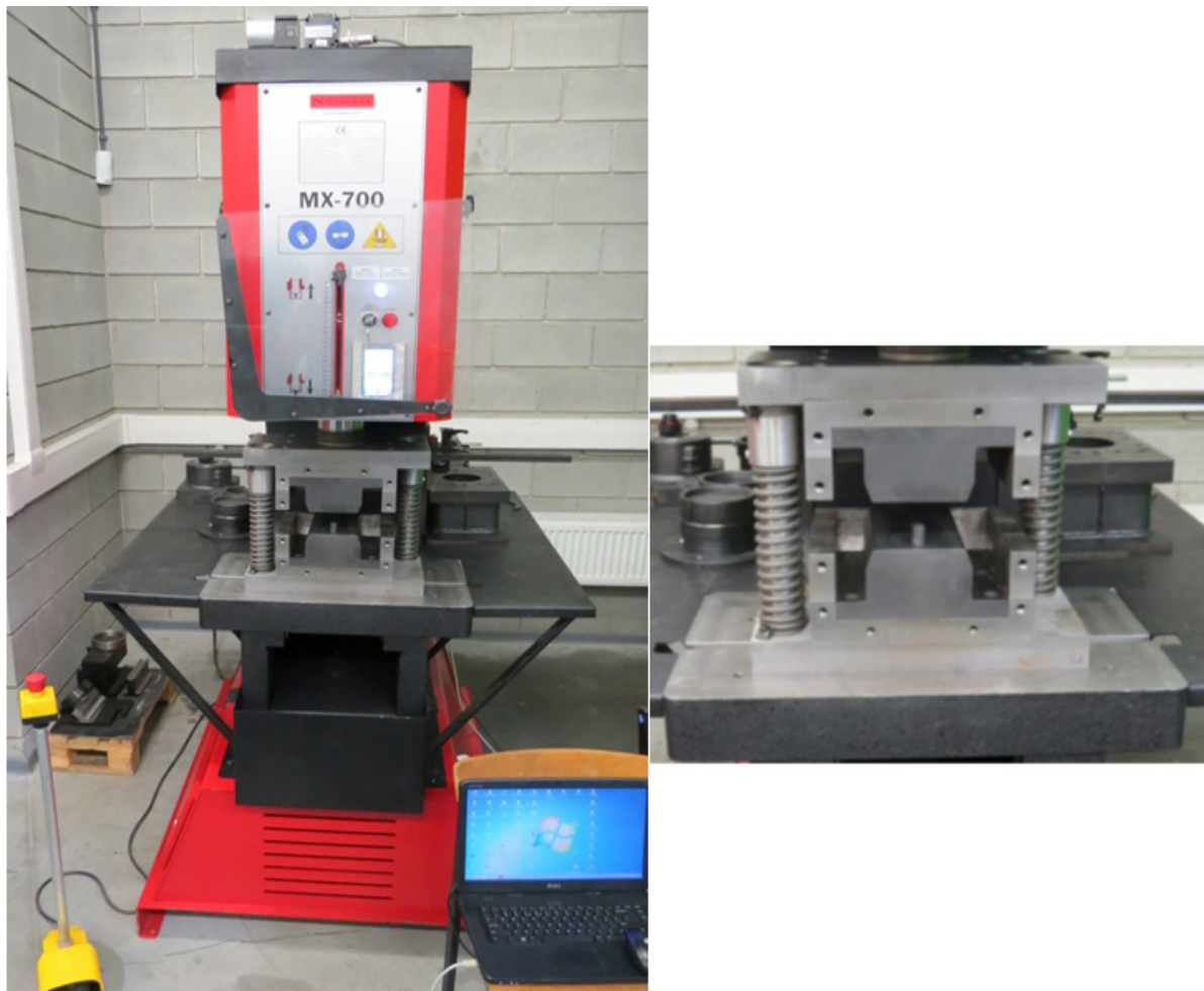
Fig. 3. Hydraulic press with upsetting device
