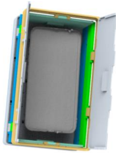
Fig. 5. Scanned mobile phone in UV-C disinfection box
