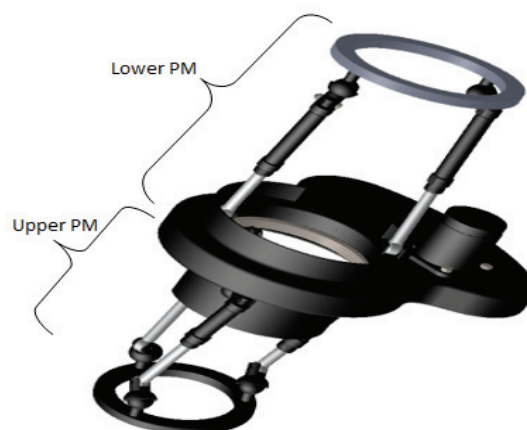
Fig. 1. 3D model of the serial-parallel robotic arm
