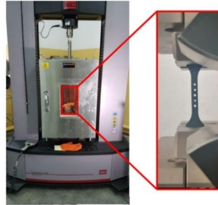
Fig. 5. Example of the specimen during the tensile test at 50°C
