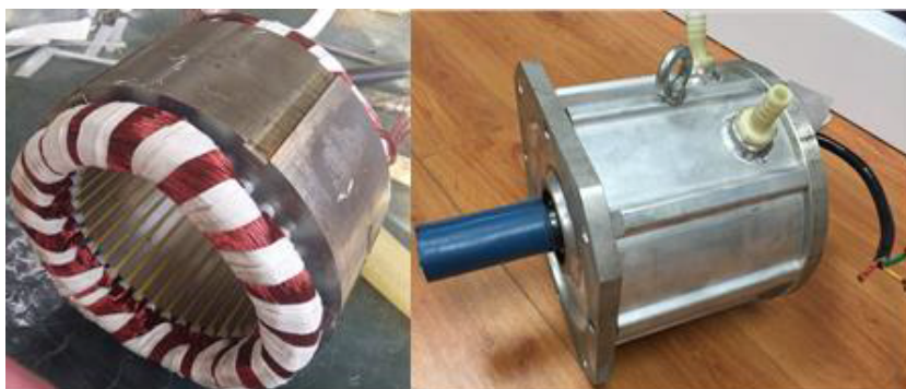
Fig. 2. Winding structure and prototype of water-cooled PMSM
