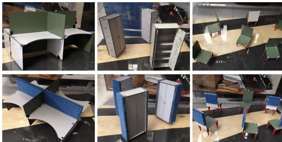
Figure 1. Scaled samples of room furnishings with (top) and without (bottom) the reference material on the selected surface: office desks, wardrobes, chairs, from top to bottom.
