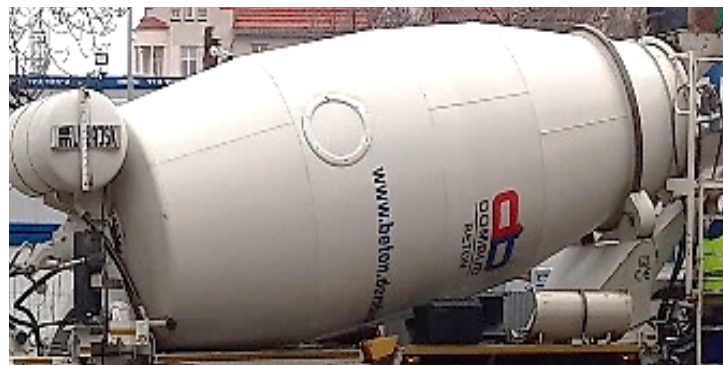
Fig. 3. A drum truck mixer after regeneration repair (own research)
