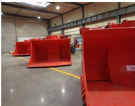
Fig. 2. Backhoe loader components made of Hardox steel (own research)
