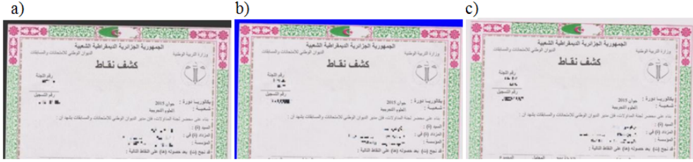
Figure 4. Detection and elimination of marginal noise: a) original AHST; b) marginal noise detected in blue; c) marginal noise removed
