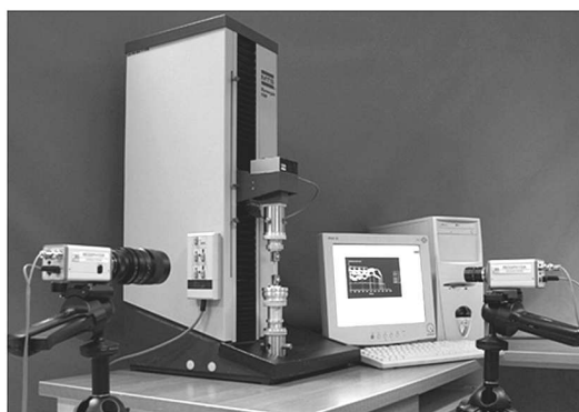
Fig. 1. Measurement set-up: testing machine ( Synergie 100 , MTS) and videoextensometer ( ME 46-350 , Messphysik )
