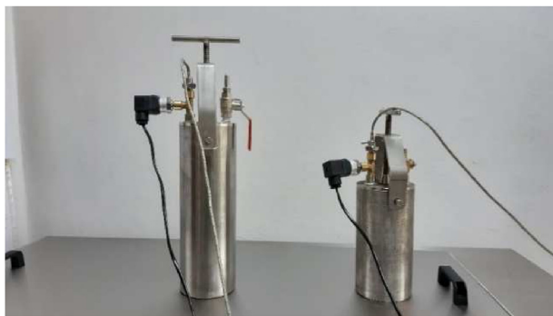
Fig. 2. Hermetic containers for core sampling in the United States Bureau of Mines (USBM) method.
