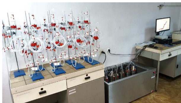
Fig. 4. Laboratory of Gas Analyses of the Central Mining Institute – the stand for methane-bearing capacity testing using the United States Bureau Of Mines (USBM) method.
