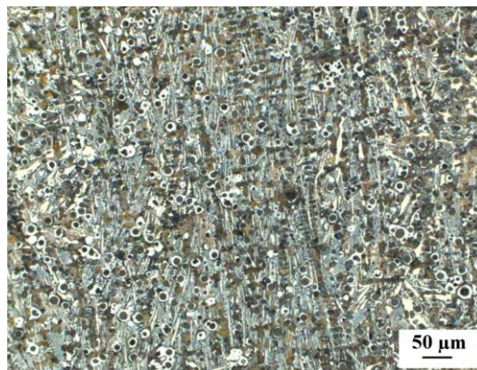
Fig. 1. Microstructure of cast iron used in the test, metallographic specimen etched in the Mi1Fe reagent (4% Nital), LM, microscope magnification 200x
