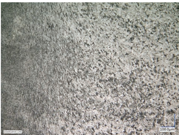
Fig. 5. Structure revealed on the martensitic steel side after etching using only Adler's reagent; on the left, a fine-grained martensitic thermo-plastic zone close to the weld line [photo: M. Ostromęcka]
