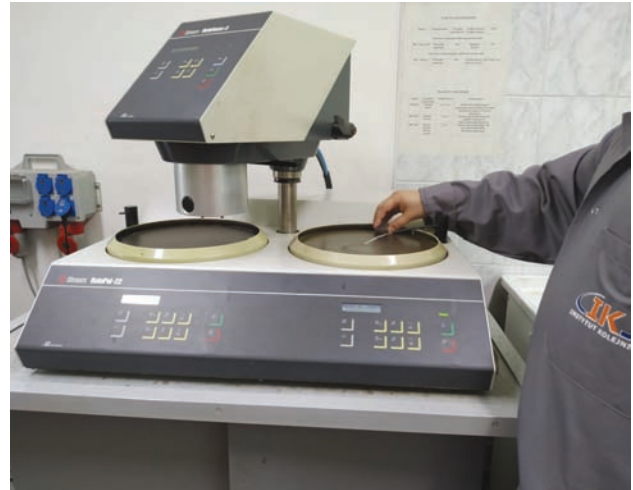
Fig. 2. Grinding on a RotoPol-22 grinding/polishing machine of Struers mould in the Materials & Structure Laboratory of the Railway Research Institute [photo: M. Ostromęcka]
