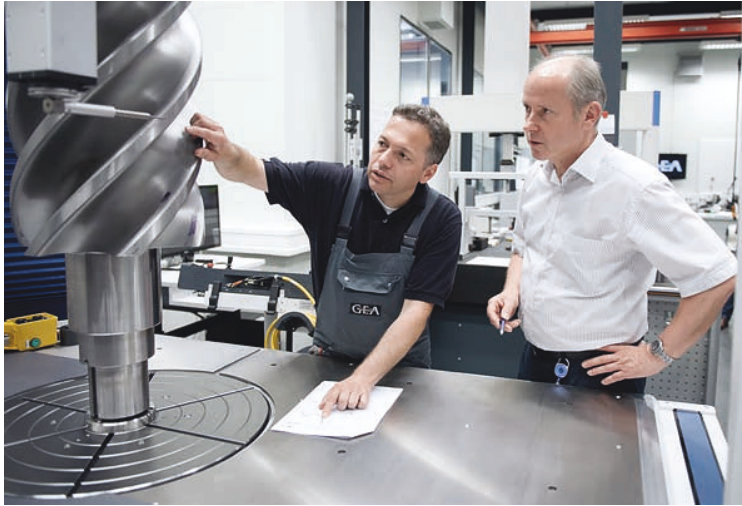
Fig. 6. Carsten Göbel and Harald Wilke discuss the measurement of a rotor on the ZEISS MMZ in the GEA Refrigeration Germany measuring lab
