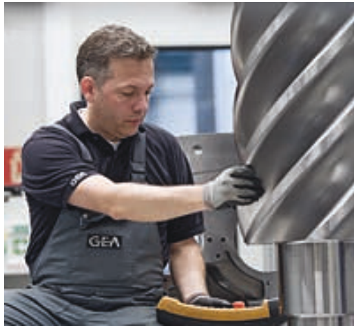
Fig. 4. The measuring technician easily places a 750 kilo-gram rotor on the rotary table of the ZEISS MMZ T
