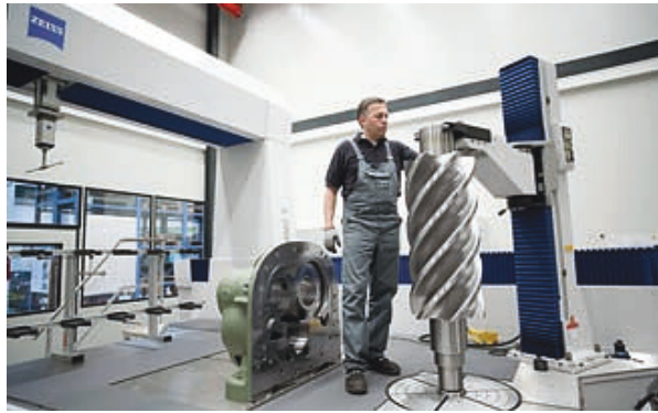
Fig. 7. The measuring technician checks the position of the rotor on the MMZ. The tailstock developed by ZEISS for GEA Refrigeration Germany reliably holds the rotor in place on the rotary table
