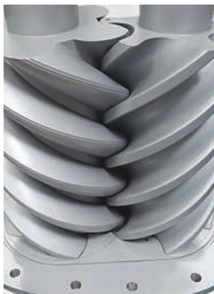
Fig. 2. The screw-shaped rotors are the centerpiece of the screw compressors which compress the gas
