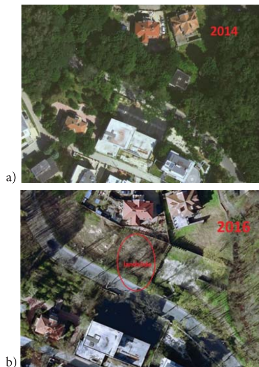
Fig. 7. Changes in the stand of trees within the landslide, which occurred between the years 2014 and 2016, (Aerial photographs shot by MGGP AERO)
