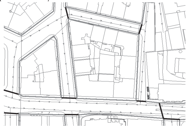
Fig. 2. Representation of sidewalks along the streets (grey) and crossings (black) in the model [own study]
