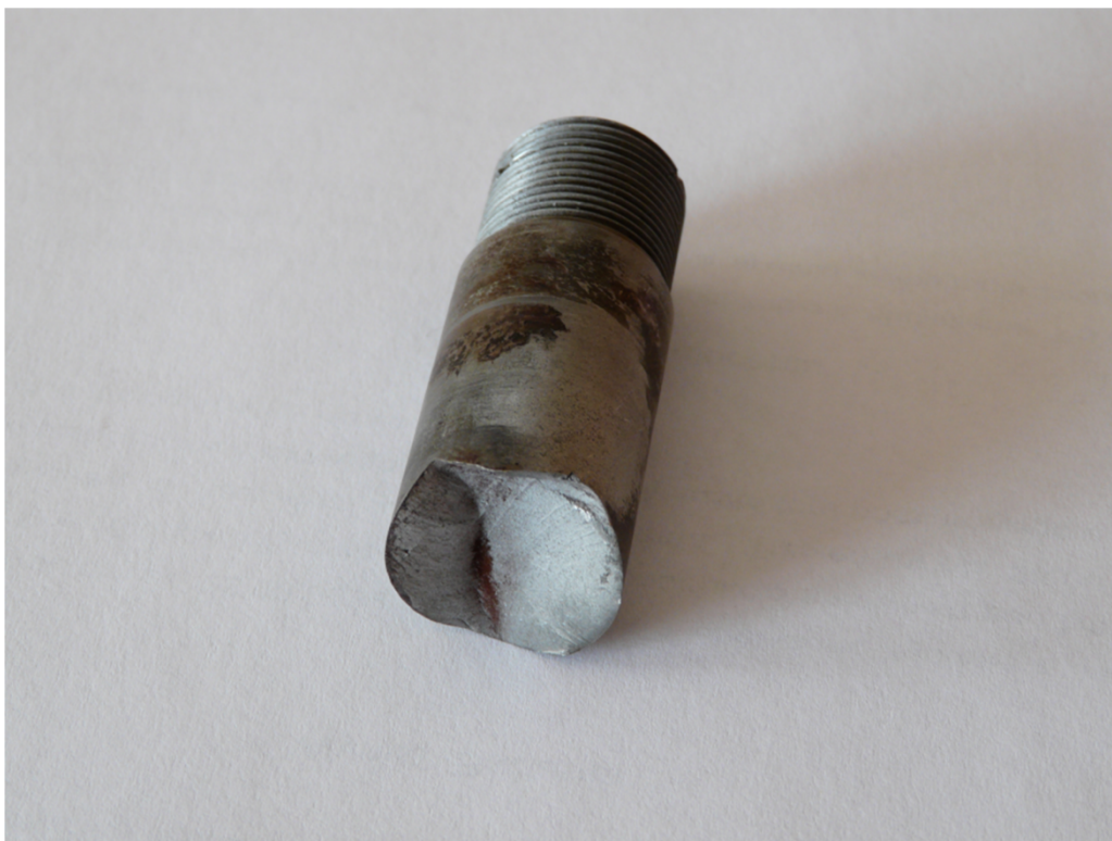
Fig. 3. Fatigue test of the PZL M28 05's wing and wing load carry-through structure. A fatigue- damaged bolt of the test fixture.
