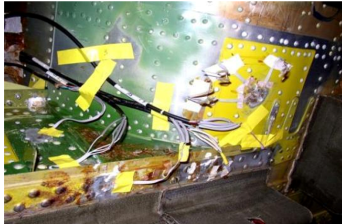
Fig. 5. Fatigue test of the PZL M28 05's wing and wing load carry-through structure. Two almost symmetrically located strain gauges on the tested article, B2-3/P and B2-3/L maximum values recorded at each of 100 flights are shown. B2-3/L indicated rising up to local damage of the tested article (see the red arrow). Repair was performed and the strain gauge was glued in approximately the same position. B2-3/P is at the undamaged side in this event (its location is shown by the yellow arrow).
