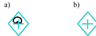
Fig. 2. AIS AtoN symbols displayed on all shipborne navigational systems and equipment [own study]: a) AIS Based AtoN, Real Position of Charted Object, b) AIS Based AtoN, Virtual position
