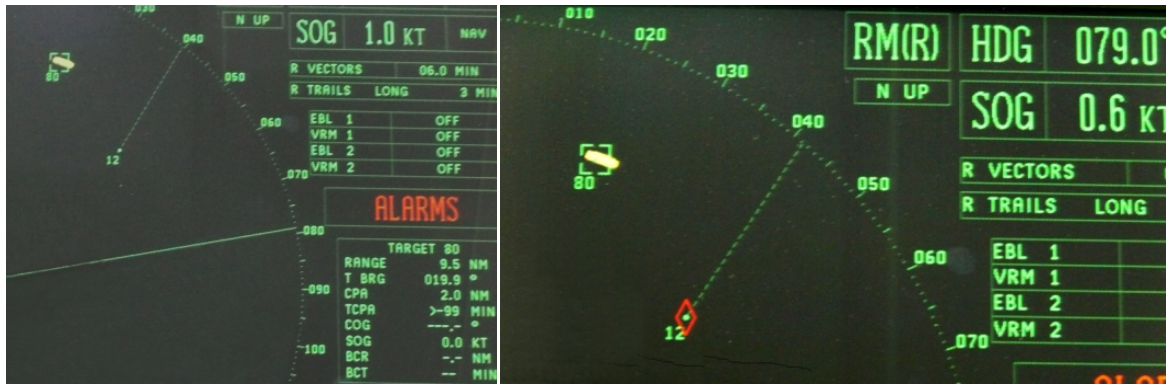
Fig. 9. Radar echo from oil platform A6A [own study]
