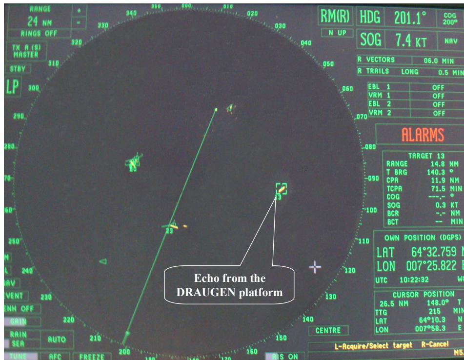
Fig. 3. Radar echo of the DRAUGEN oil platform [own study]
