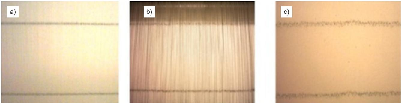
**Figure 2.** Photographs of reference grids on the fabrics. The distances measured: a) on the warp beam, b) on the front of reed c) on the fabric when loom is working.
