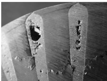
Fig. 4. Tested motor with damaged rotors (a) and a sample of bad made bar of cage (b)
