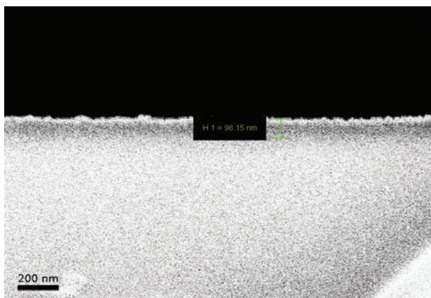
Fig. 15. Imaging with the mass contrast EsB detector shows that the AlN layer on a glass slide is ca. 100 nm-thick after 625 deposition cycles.
