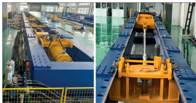
Fig. 1. Structural diagrams of 3000-t and rope-tension-reciprocating testing machine
