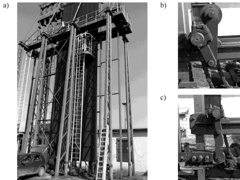
Fig. 9. Test stand: a) general view, b) initial and c) final position of the beater
