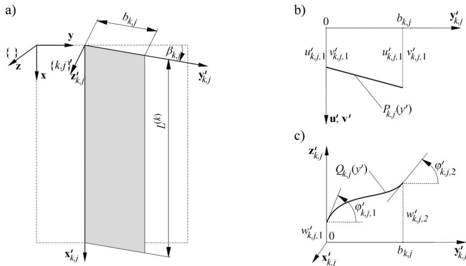
Fig. 7. Models of displacements of strip  $j$  of electrode  $k$  : a) coordinate system  $\{k, j\}'$ , b) nodal displacements  $u'_{k,j,1}, v'_{k,j,1}, u'_{k,j,2}, v'_{k,j,2}$  – polynomial  $\mathbf{P}_{k,j}(y')$ , c) nodal displacements  $w'_{k,j,1}, \varphi'_{k,j,1}, w'_{k,j,2}, \varphi'_{k,j,2}$  – polynomial  $\mathbf{Q}_{k,j}(y')$
