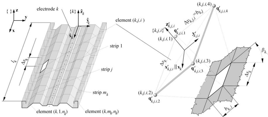
Fig. 4. Strip  $j$  with width  $b_{k,j}$  and angle of inclination  $\beta_{k,j}$  towards axis  $\hat{y}$ ,  $\{\}$  – global coordinate system,  $\{k\}$  – local coordinate system connected with electrode  $k$  with axes parallel to those of system  $\{\}$
