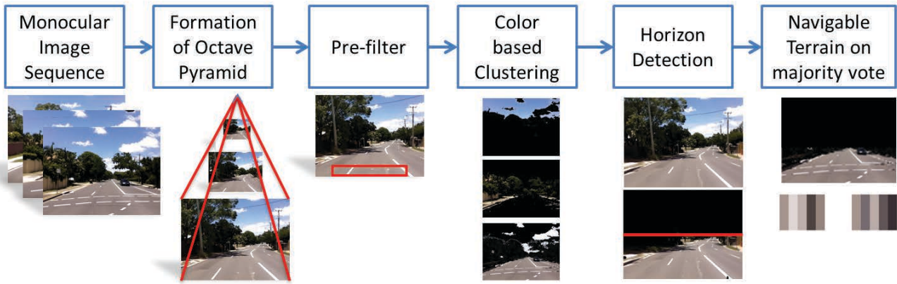
Figure 2. An overview of the algorithm – with individual stages and their corresponding outputs. The processing pipeline is sequential and each stage enables parallel processing at the pixel level.
