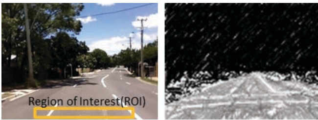
Figure 5. Pre-filtering based on the Region of Interest (ROI), highlighted in orange. The image on the right are pixels which fall within one standard deviation of ROI mean.
