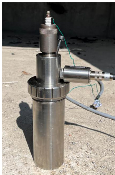
Figure 5. Manometric bomb with test igniter
