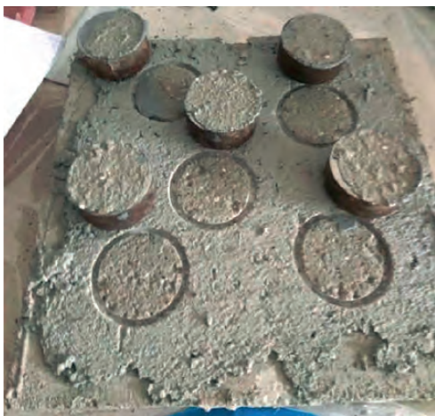
Fig. 8 Discs detached from the concrete surface with cuts
