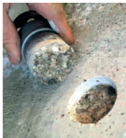
Fig. 3. Correctly performed adhesion measurement using the pull-off method [14]
