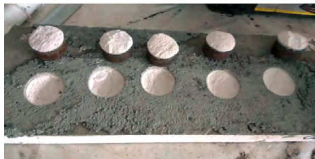
Fig. 7. Discs torn off from the aerated concrete surface with cuts
