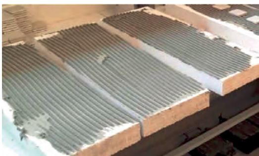
Fig. 5. Preparation of samples for adhesion tests – mortar application
