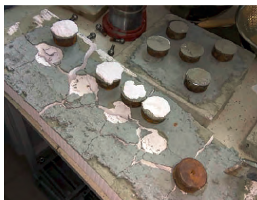
Fig. 6. Metal discs torn off on the surface of the plates
