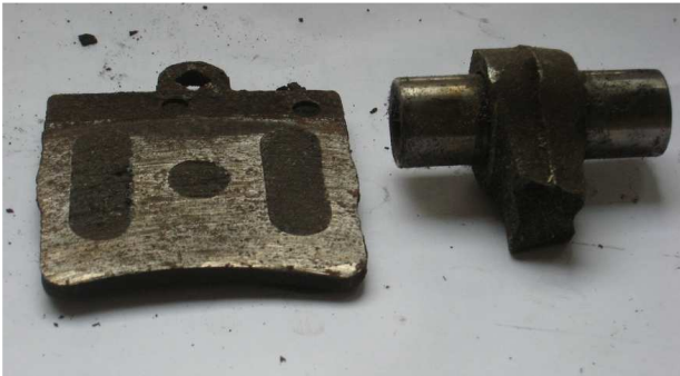
Figure 6. Example of wear-out failure (brake shoe – to the left) and sudden disruption (connecting-rod – to the right)
