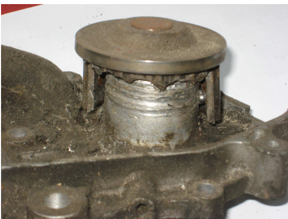
Figure 8. Total, secondary destruction of water pump (car engine) due to primary bearing failure
