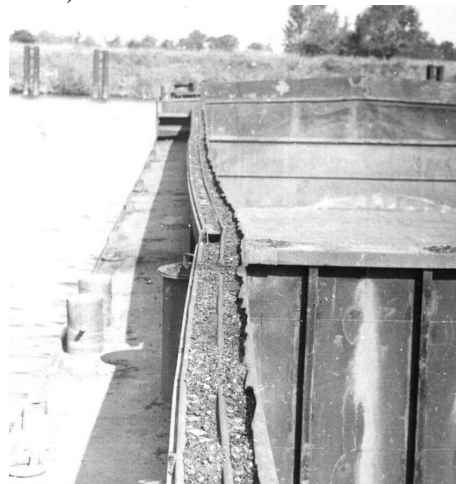
Figure 10. Example of macro notch of deck transom of river barge BP-500
