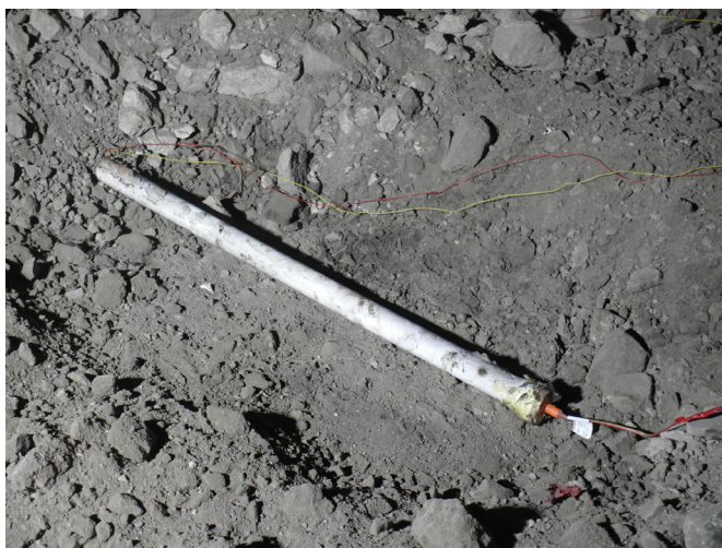
Figure 3. The test sample of bulk emulsion explosive in a sewage pipe
