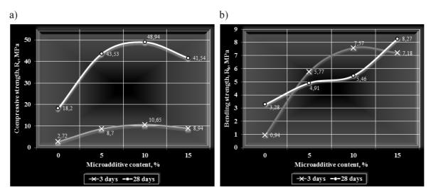
Fig. 2. Tensile strengths of the fine-grained concrete depending on the microadditive on the basis of silica sand content: a) under compression, b) under bending
