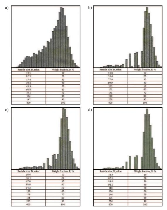
Fig. 1. Diagram of the grains distribution: a) silica sand, b) silica sand + additive S-3,c) silica sand + calcium stearate, d) silica sand + additive S-3 + calcium stearate
