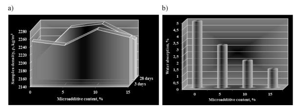
Fig. 3. Dependence of the fine-grained concrete samples from the content of the integrated organic-mineral additive: a) density, b) water absorption
