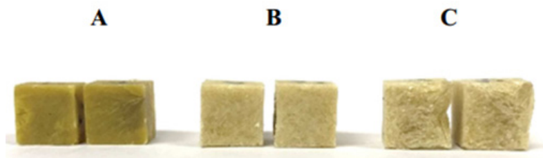
Figure 4. Images of pellets post temperature cycling for >100 cycles of: A – DNAN doped with 5 mol% ‘EDX-1’, B – \alpha -DNAN, and C – \beta -DNAN [60]
